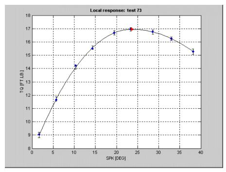
To model responses that are characterized in appearance by a single and well-defined stationary point with asymmetrical curvature either side of the local minimum or maximum, define the following spline class,
