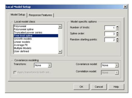
A spline is a piecewise polynomial, where different sections of polynomial are fitted smoothly together. The point of the join is called the knot.
