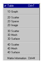
The Design Evaluation tool has options for 1D, 2D, 3D, and 4D displays. You can switch to these by clicking the toolbar buttons or using the **View** menu.
